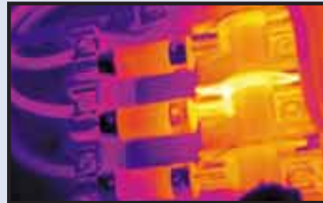
Poor clip connection on center fuse
